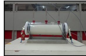
Figure 5. Thermocouple positioning
