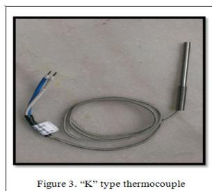
Figure 3. "K" type thermocouple
