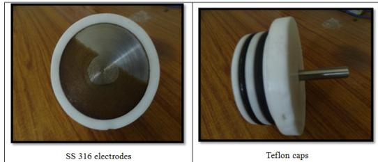
Figure 2. Electrodes of ohmic heater
