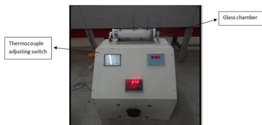
Figure 6. Experimental setup of ohmic heating
