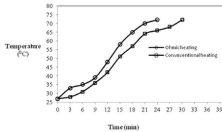
Figure 1. Comparison of temperature histories for ohmic heating and conventional heating at each set temperature.
