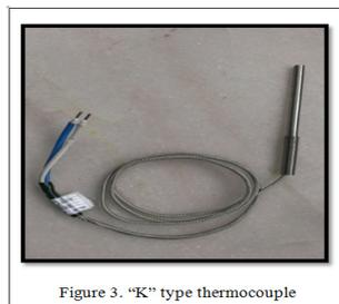
Figure 3. "K" type thermocouple
