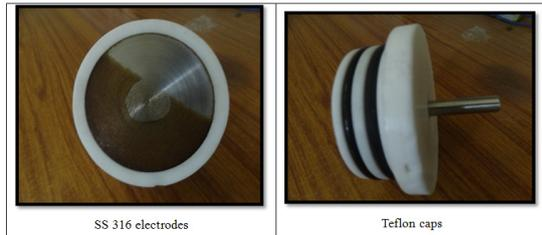
Figure 2. Electrodes of ohmic heater
